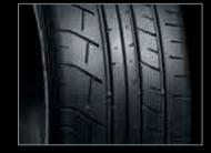
Even the design details of the GT-R's Dunlop SP Sport MAXX GT600 DSST CTT high-performance run-flat tyres are obsessive: a tiny block of rubber added to one of the treads combats tread squirm and gives a more confident, precise feel at the wheel.
