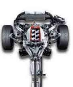
Dry Sump Lubrication System To ensure stable lubrication for the transmission even when cornering at high Gs, a dry sump lubrication system is employed. The system sprays transmission oil directly onto the gears, reducing friction and increasing reliability.
